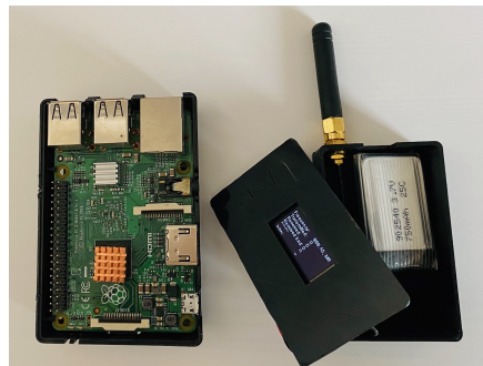
Fig. 4. Opened DTN pager device with a Raspberry Pi for size reference.
